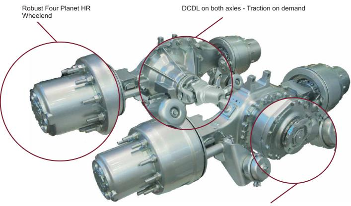
Needle Roller bearings and optimized driveline angle for long life & reduced NVH
