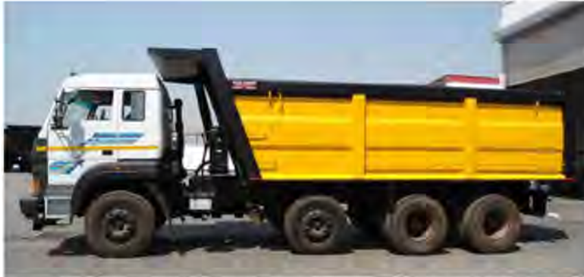
The two-speed axle will boost the appeal of presently niche applications such as this 8×2 construction tipper by Black Diamond Motors on Tata 3118 chassis.
